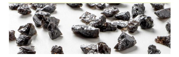
BROWN FUSED ALUMINIA is a non-disposable abrasive according to DIN EN ISO 11126-7 N/FA-A/G and is based on aluminium oxide.
